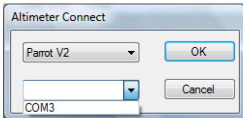
Select the correct altimeter model and the comm port to which the Raven is connected. If multiple comm ports show up in the dialog box, the highest-numbered one will probably be the one with the Raven connected to it.
