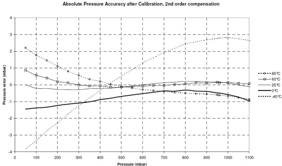
The Raven uses the 2<sup>nd</sup> order compensation referred to above, resulting in less than 1 mbar (0.1% full-scale) pressure error over most conditions, and less than 3 mbar pressure error (0.3%) the temperature range from -40C to 85C, and from 1.1 Atm (2500 feet below sea level) to 0.05 Atm (70,000 feet above sea level).
