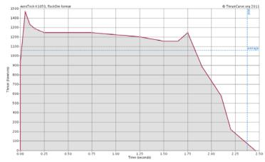
This thrust curve for the Aerotech k1050 shows an almost optimal burn pattern for how heavy our rocket is. It gives a nice fast boost off the pad, and then holds a steady burn until it gives one last bump of power at the end for a nice stead flight and a smooth arch at apogee.
