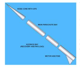
The Rocket was designed using Rocksim and is made up of 4 main parts. First there is the 24 inch long conic nose cone with a 6 inch long shoulder. There is a ½ inch thick plywood bulkhead (laminated with 1/8 inch thick G10 fiberglass on the lower end for added strength) at the top of the nosecone shoulder. This is where the shock cord attaches to. The nosecone is attached to the upper section via 3 #2 sheer pins. Next is the 56 inch upper section that holds our 32
