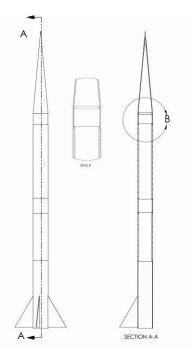
inches, a semi span of 7 inches, and they will be 0.1875 inches thick. The fins are made entirely out of G10 fiberglass.
