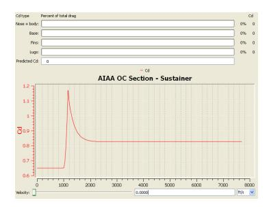
This is a graph that shows our CD compared against velocity (in ft/s). Up until Mach we have a low CD of around .65. We found this value very suitable, as it is an average value, and possibly slightly low for a 5 inch diameter rocket. We were not
