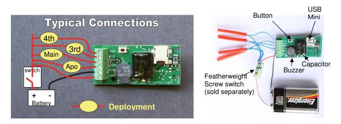
A description of the default program for the 4 outputs is given in the <u>deployment</u> <u>programming section</u> of this document.
