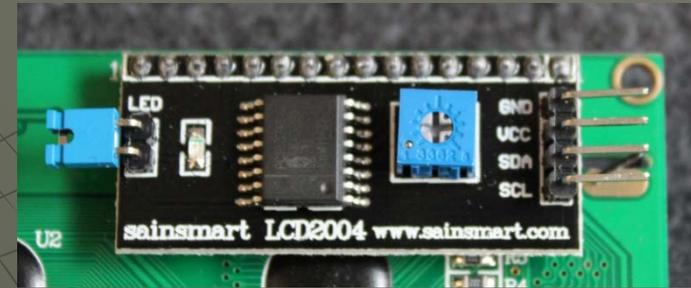
The Sainsmart LCD2004 20x4 I2C module uses the HD44780 controller from Hitachi and a PCF8574 I2C 8 bit I/O expander
