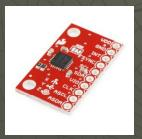
3 Axis Accelerometer & Gyro (~\$40) Sparkfun: https://www.sparkfun.com/products/11028
