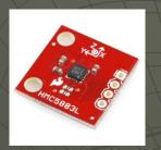
3 Axis Magnetometer (~\$15) Also used on S4
