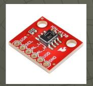
Humidity and Temperature Sensor (~\$30) Also used on S4
