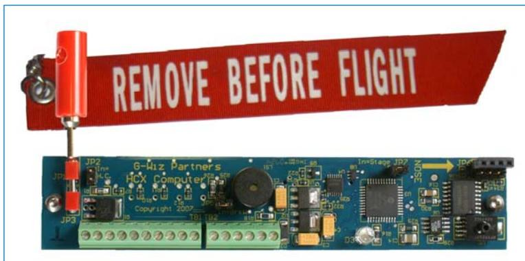
hole in the airframe, the built-in shunt is the most practical method to safe your pyro ports. When the shunt plug is properly installed, connecting JP1 and JP3, it protects the pyro ports from accidentally firing.
