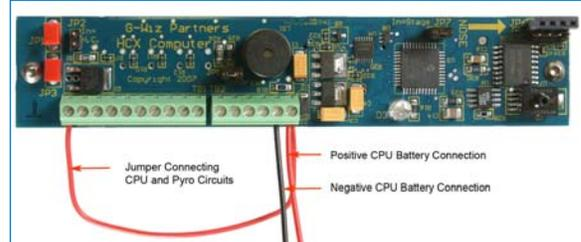
**Note:** You must have power on the flight computer in order to connect it. Wire up your flight computer in single battery mode before you attach it to your personal computer. This is a picture of the flight computer in simple single battery mode. While you do not need to attach the jumper wire between the CPU and the pyro circuit, we recommended you do so because otherwise you will get a (very annoying) low battery warning.
