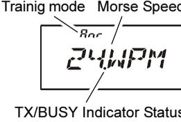
5. Rotate the **DIAL** knob to select the Morse speed. You may select the units of the code speed between “WPM (Words per minute)” and “CPM: characters per minute)” by pressing the **[V/M(DW)MT]** key.
