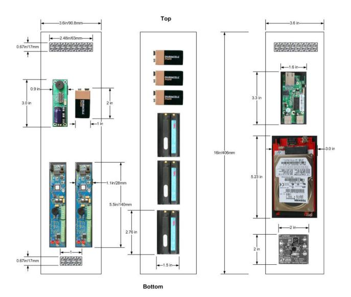
This Visio drawing of the avionics bay shows the dimensions of all the components that are to be secured onto the sleds. The right-most sled is the top of the payload sled, the middle sled is the bottom side of the recovery sled, and the left-most sled is the top side of the recovery sled.
