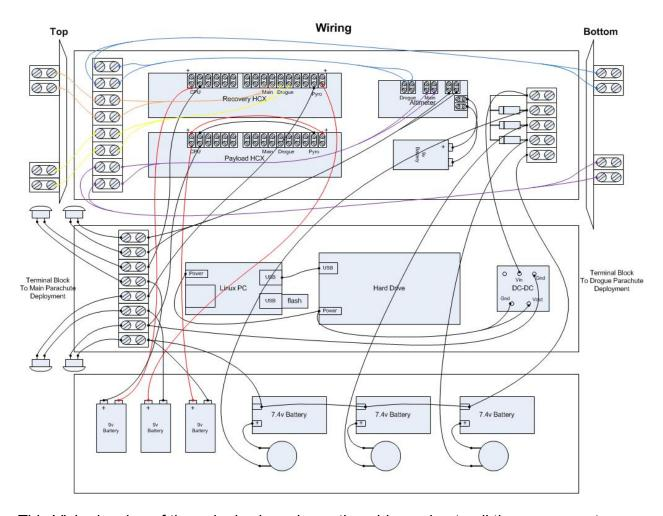
This Visio drawing of the avionics bay shows the wiring going to all the components in the avionics bay. The top sled represents the top of the recovery sled, the middle sled represents the top of the payload sled, and the bottom sled is the bottom of the recovery sled
