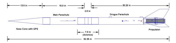
The vehicle was constructed of the same G-10 material as the full sized model with a scaled avionics bay. The vehicle can be flown with engine ejection and a single main parachute in place of the drogue, or with dual recovery with a drogue parachute as well as a main parachute.
